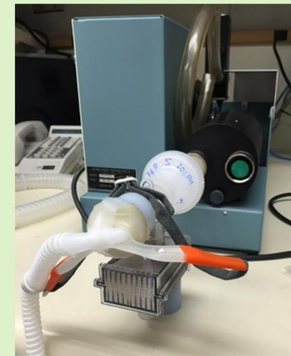
Figure 4. HFNC prongs attached to simulated nares connected to Harvard Lung machine.
